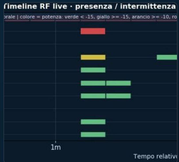
Timeline view showing cellular uplink presence, recurrence and power-coded segments.
