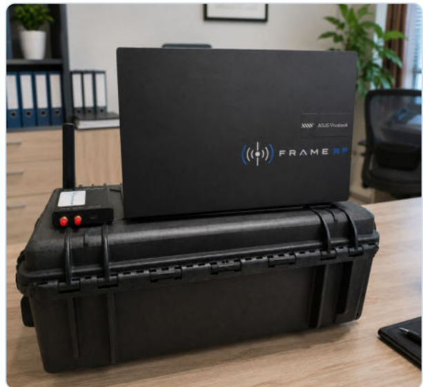
Portable workstation with SDR and antenna, prepared as a field-ready FRAME RF setup.
